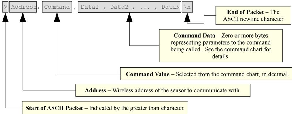
**Figure 4 - Chain ASCII Command Packet Format**
