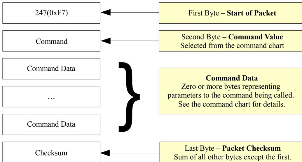
**Figure 1 - Typical Binary Command Packet Format**
