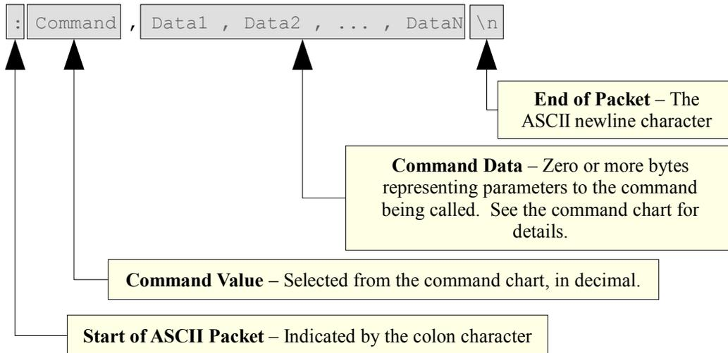
**Figure 2 - Typical ASCII Command Packet Format**
