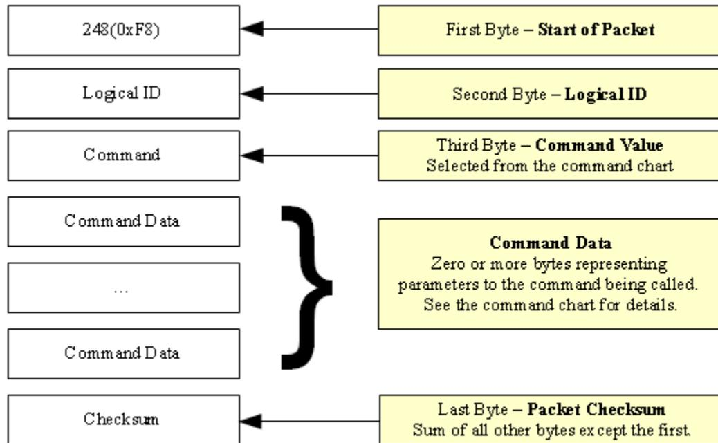
**Figure 3 - Chain Binary Command Packet Format**
