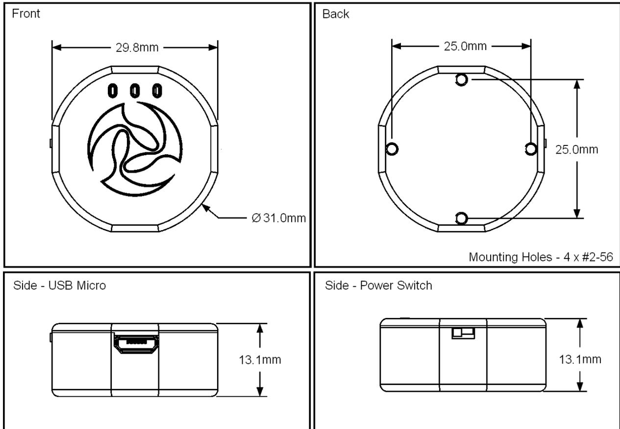
The Yost Labs 3-Space Mini Bluetooth is packaged as a 29.8mm x 29.8mm x 13.1mm casing with 3 indicator LEDs, a Micro USB 2.0 port, and power switch on the side. There are four mounting holes on the bottom for use with #2-56 screws.
