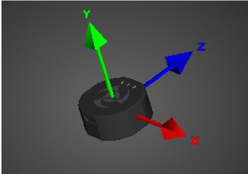
Bear in mind the difference between natural axes and the axes that are used in protocol data. While they are by default the same, they can be remapped so that, for example, data axis Y could contain data from natural axis X. This allows users to work with data in a reference frame they are familiar with.
